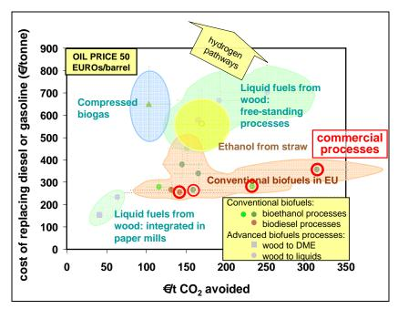
Fig. 1: Cost of replacing fossil fuel and of reducing CO<sub>2</sub> emissions
