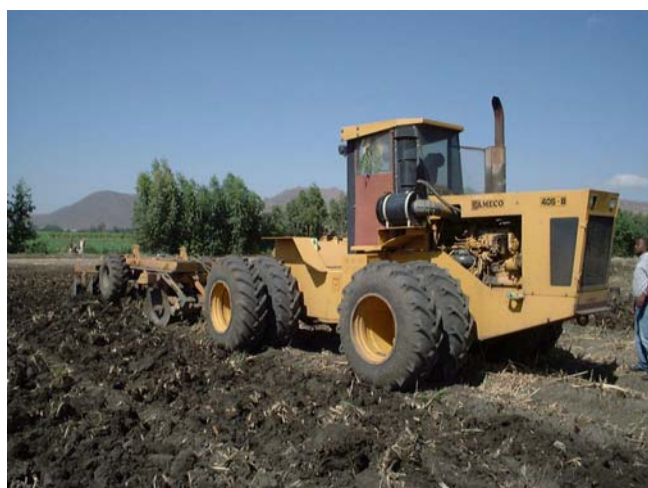
Heavy wheeled tractor with disc plough/harrow. Booker Tate Ltd.
