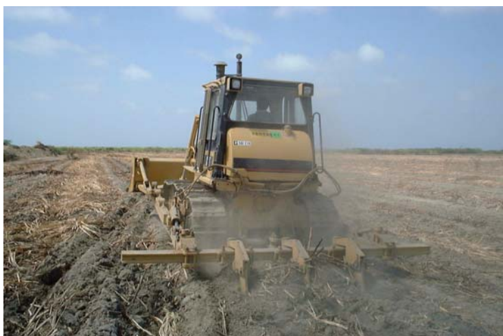
Heavy crawler tractor deep ripping. Booker Tate Ltd.
